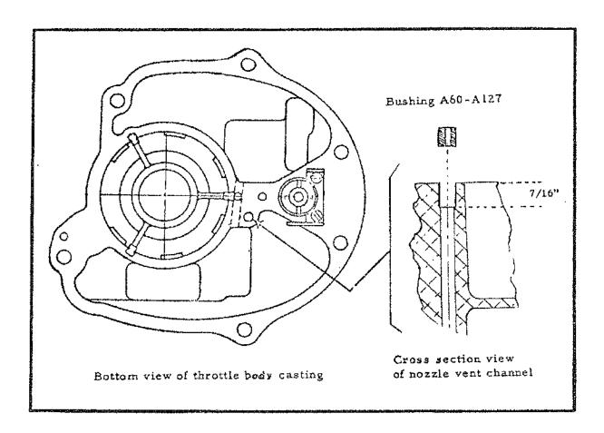
Very carefully counterbore this channel to a depth of 7/16" using the #9 drill. Clean out all chips after drilling (clean this channel by removing the economizer plug and blow out with compressed air with the throttle valve in a closed position).
